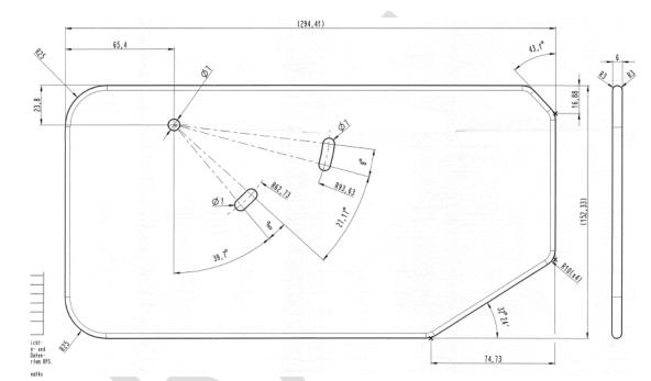
2 side plates (WSC delivery or Specific parts); All edges will be rounded with at least R3mm (Safety)
